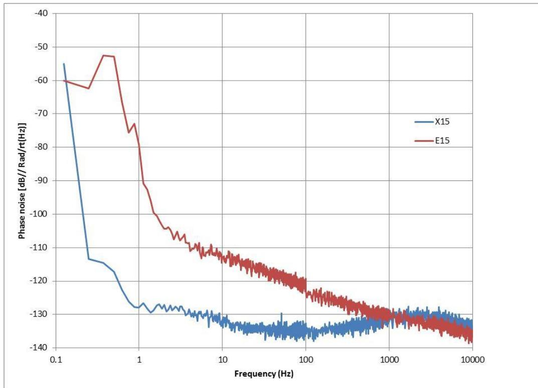
**Figure 2: Phase noise of the Koheras E15 and X15 laser modules. Plots are normalized to an optical path imbalance of 1m.**
