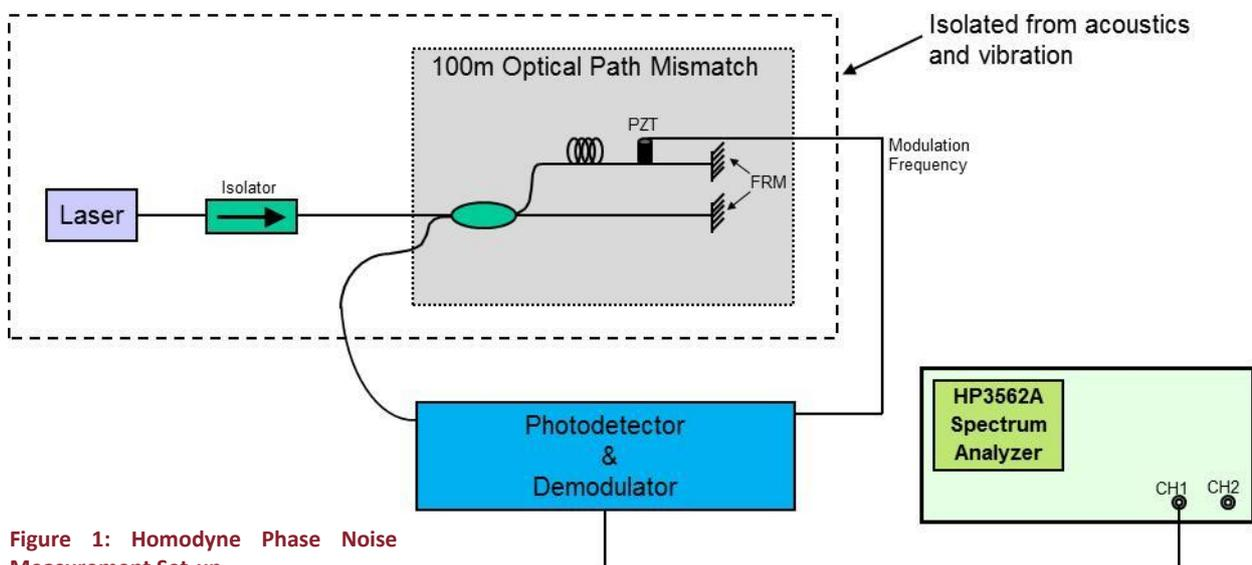
**Figure 1: Homodyne Phase Noise Measurement Set-up**
