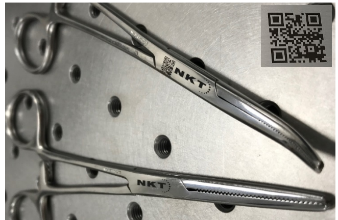
Logos and data matrix marked on stainless steel forceps and scissors
