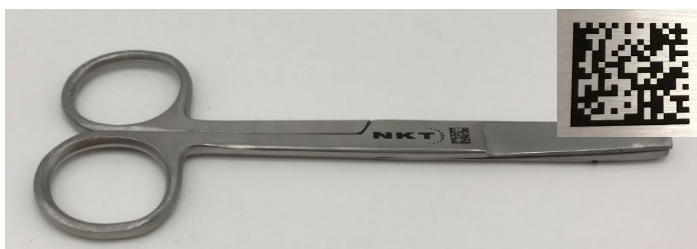
Laser marking has rapidly become the preferred UDI marking process
