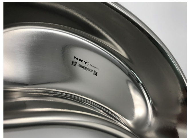
Logo and barcode marked on stainless steel kidney dish
