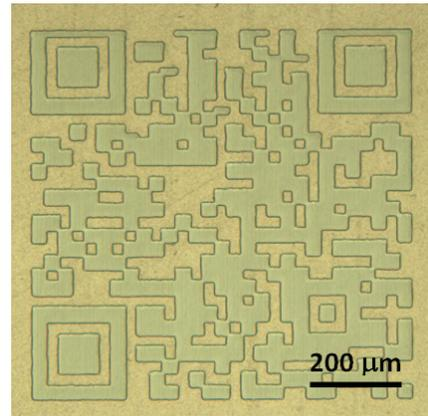
**Microscope image of a patterned area of TCO. The image demonstrates the capability to selectively remove and pattern the TCO layer in arbitrary and complex shapes.**
