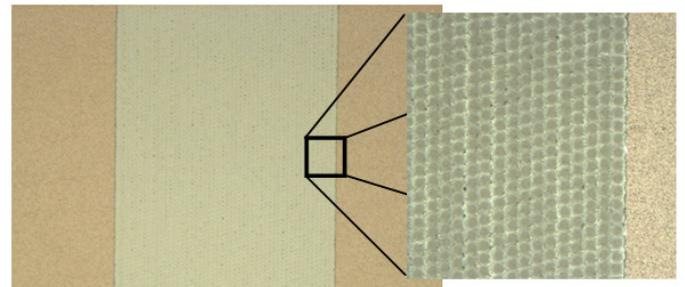
**Microscope image of an area cleared of the TCO layer. The image demonstrates the capability to cleanly remove large areas of TCO that are fully insulating.**
