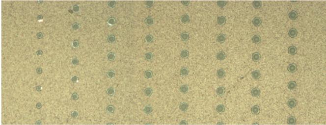
**Microscope image of scribes of increasing pulse energy (from left to right). The lines sequentially increase in power to the right and each creates an increasingly large mark.**
