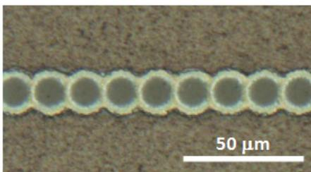
**Reflection microscope images of scribes in FTO TCO back-contact thin-film PV devices using relatively high and low power levels to demonstrate the ability to remove TCO and buffer layer or to selectively remove the TCO layer only.**
