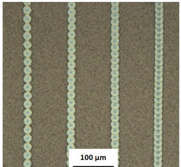
Linear scribes of a FTO thin-film TCO on a glass substrate made with Fianium's high energy picosecond fiber laser.
