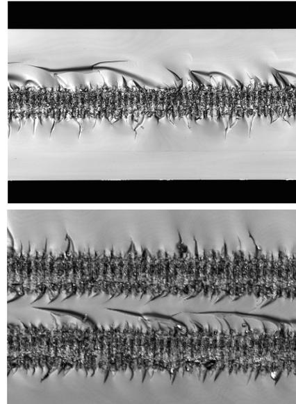
**Figure 3.** Microscope images of the break edge of 100  $\mu$ m thick (top) and 330  $\mu$ m thick (bottom) sapphire wafers. The wafers were internally scribed and the thicker wafer was double scribed for an easier and more reliable break.
