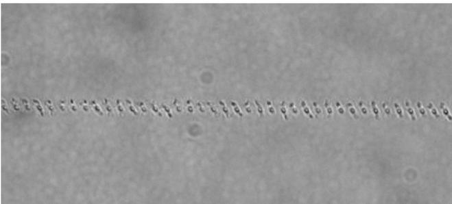
**Figure 2.** Transmission mode optical microscope image of an internal scribe in display glass.
