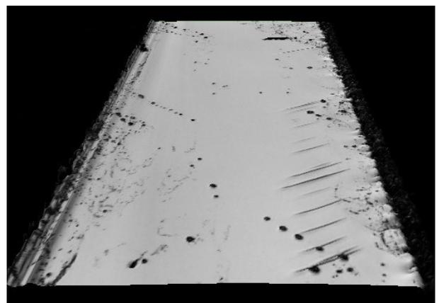
Height map (top) and intensity (bottom) 3D images of the break edge of a 330  $\mu$ m thick Sapphire wafer scribed on the surface with one of Fianium's high energy picosecond fiber lasers.
