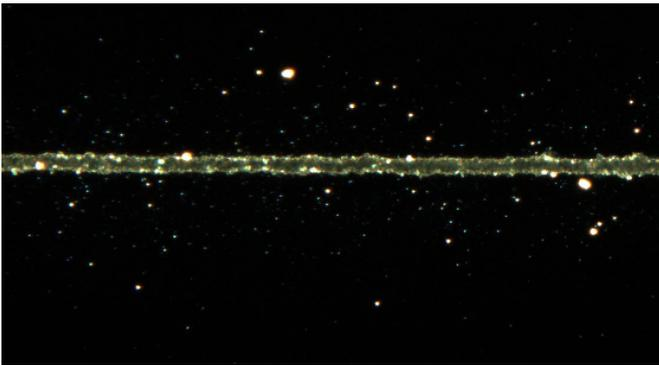
**Figure 1.** Dark field microscope image of a surface scribe of a sapphire wafer.
