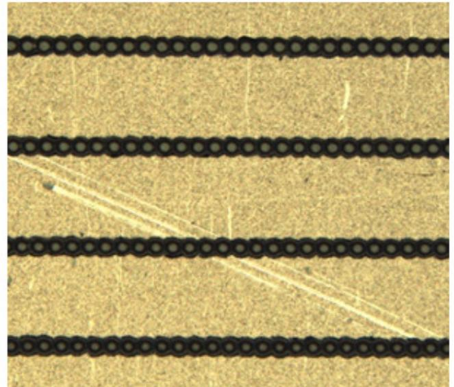
Multiple P3 scribes each separated by 200  $\mu\text{m}$  demonstrate the quality and repeatability of picosecond laser scribing of thin-film PV devices. The scribe power is varied by over 40% from top to bottom, which demonstrates the broad processing window.
