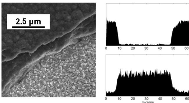
SEM image of the scribe channel sidewall (left) demonstrates a sharp edge with no heat-affected zone and an undamaged underlying TCO. X-ray EDS data across the width of the scribe channel (right). The image on the top-right is the silicon signature and the bottom right is the TCO signature.
