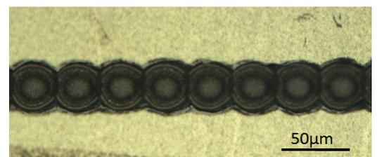
Microscope images of P2 (top) and P3 (bottom) scribes on an amorphous-Si thin-film photovoltaic device. The scribes were made with a high energy picosecond fiber laser from Fianium at rates of over 3000 mm/s. The scribes show complete removal of the a-Si absorber and metal back-contact layers with no damage to the underlying TCO.
