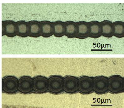
Microscope images of P2 (top) and P3 (bottom) scribes on an amorphous-Si thin-film photovoltaic device using the Fianium HE1060/532 picosecond fiber laser. The scribes show complete removal of the a-Si absorber and metal back-contact layers with no damage to the underlying TCO. The process speed was over 3000 mm/s for both scribes.
