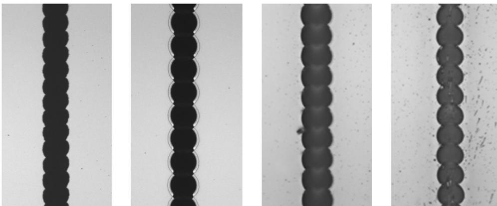
Scribes of molybdenum thin films on glass created using various picosecond and nanosecond fiber lasers. The pulsewidths are 3ps, 46ps, 10ns, and 100ns from left to right. Significant heat-related defects, such as melting and chipping, are observable in the nanosecond results, while the picosecond scribes are fully defect-free.
