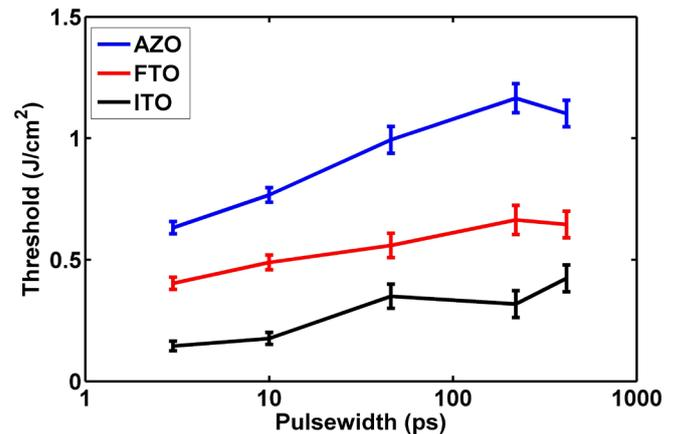
Transparent conducting oxide (TCO) film removal thresholds as a function of laser pulsewidth for three TCO types of various thicknesses. Required pulse energy for film removal is observed to increase with pulsewidth.
