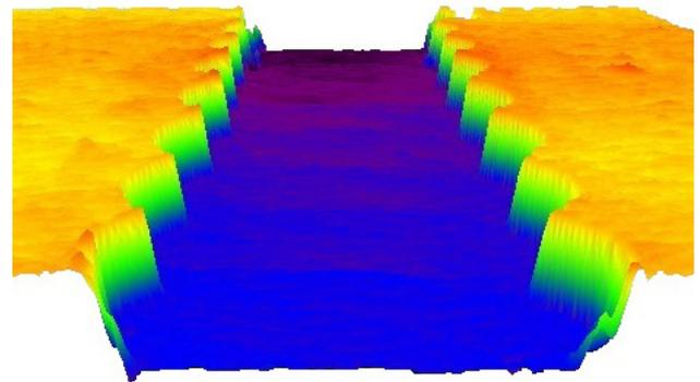
3D image of molybdenum metal film on glass selectively removed using a picosecond fiber laser from Fianium
