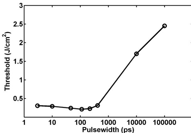
Molybdenum film removal threshold as a function of laser pulsewidth. Threshold is mostly constant for the picosecond results, but increases by an order of magnitude in the nanosecond regime.
