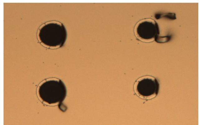
Single pulse material removal by 10ns pulses demonstrating chipping defects
