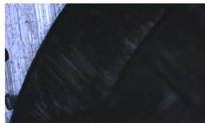
Photo of rings milled into the surface of a CFRP coupon, 250 μm deep per ring (top). Microscope image of the concentric rings (left).
