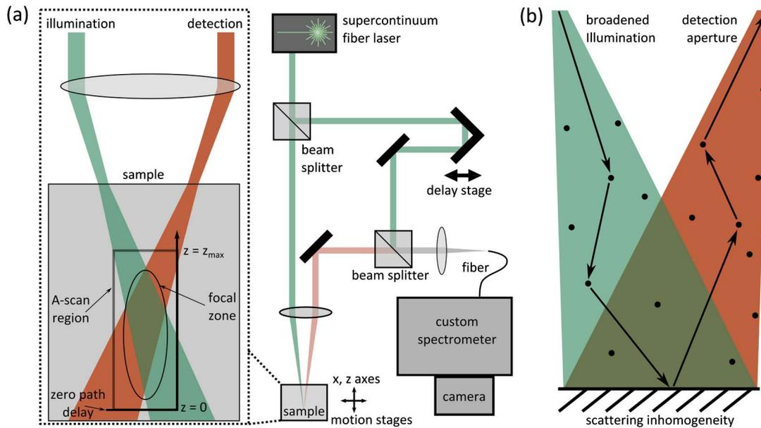
Fig. 1. (a) Diagram of system setup. The ms2/LCI instrument consists of a modified Mach–Zehnder interferometer and a custom spectrometer. The inset shows the arrangement of focal volume in the sample and the location of the zero path delay point. (b) Cartoon illustrating an example path of a multiply forward scattered photon used to image a scattering inhomogeneity.
