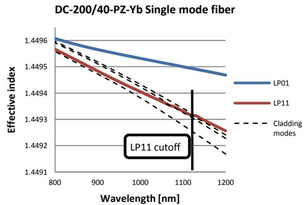
**Figure 3:** Simulated effective mode indices of the first 5 modes in a DC-200/40-PZ-Yb fiber. The LP<sub>11</sub> mode exhibits a short-wavelength cutoff at ~1120nm, and the fiber is single mode for wavelengths below. The figure refers to the transverse (x-) polarized modes. The stress applying parts induce a strong birefringence, which lowers the effective indices of the corresponding y-polarized modes, which therefore are not guided in the wavelength range shown.
