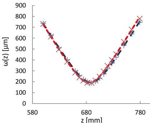
**Figure 5: Measured spot size vs. propagation distance for a collimated beam from a DC-200/40-Pz-Yb fiber. The spot size was measured both in x-direction and y-direction. The fits yield an  $M^2$  value better than 1.15.**
