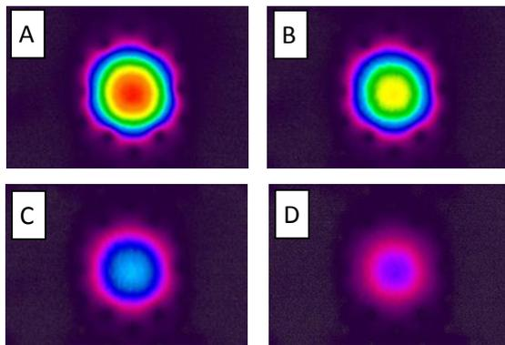
**Figure 2:** Near-field images of the fiber for optimum alignment (A) and gradually misaligned input beam (B-D). The output beam symmetry is maintained for all positions of the input beam and no higher order modes could be excited. The mode field diameter is 32 μm. The images are obtained on a CCD camera.
