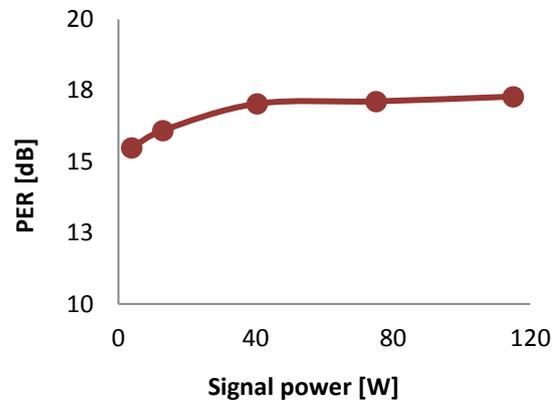
Figure 10: Measured PER as a function of signal power.
