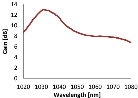
Figure 5: Calculated gain profile for the aeroGAIN-ROD-PM55.
