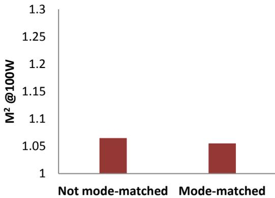
Figure 11: Measured beam quality at 100W output power for a non mode-matched seed and a mode-matched seed.
