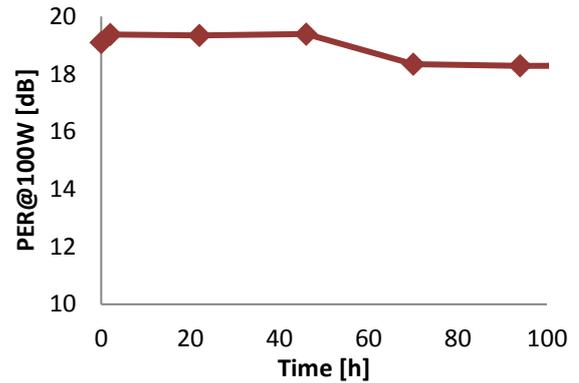
Figure 13: Measured PER over a 100 hour burn-in period.
