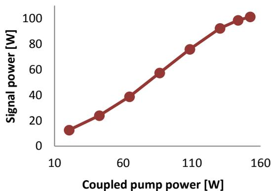
Figure 8: Signal average output power as a function of coupled pump power.
