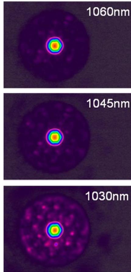
Figure 6: Near field images at three different seed wavelengths without amplification.
