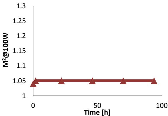
Figure 12: Measured beam quality over a 100 hour burn-in period.
