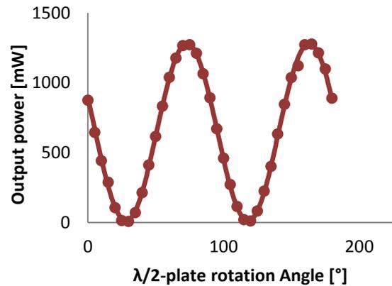
Figure 9: Output power as a function of half-wave plate rotation angle.
