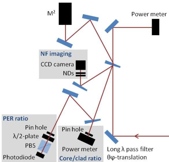
**Figure 2: Beam diagnostics for testing the aeroGAIN-ROD-PM55.**
