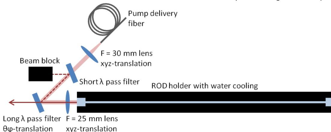
**Figure 3: Setup for pump coupling.** The pump light is coupled from a delivery fiber into the rod fiber in the backward direction using a set of high NA mode matched lenses. A dichroic mirror is used for extraction of the signal light.
