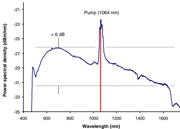
Fig. 5: Power spectral density at the end of 20m of SC photonic crystal fiber. (Pump power in the fiber: 10 mW, pulse width: 1 ns, repetition rate: ≈7 kHz. Spectrometer resolution: 5 nm)
