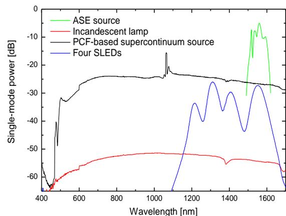
Fig. 2: Comparison of the power spectral density delivered into a single mode fiber for various broadband light sources. The SLED source contains four separate SLEDs with different centre wavelengths. The total integrated power for of these spectra are: ASE-source: 13 mW (+11 dBm), SLEDs: 160  $\mu$ W (-8 dBm), Incandescent lamp: 3  $\mu$ W (-25 dBm) and Supercontinuum source: 2 mW (+3 dBm)
