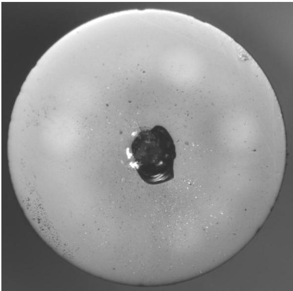
**Figure 4: End view of a damaged facet**
