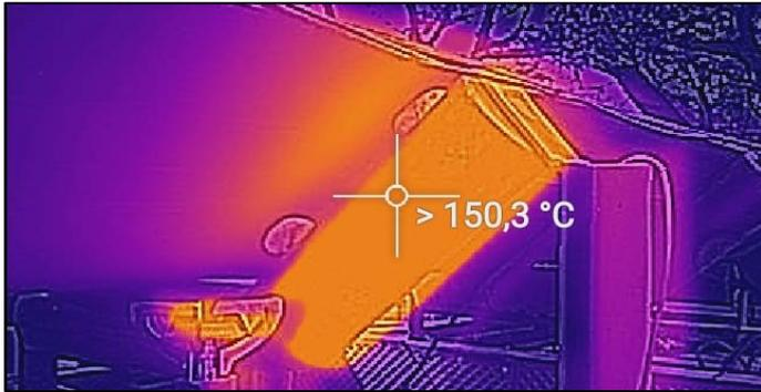
Figure 8. Temperature of idler just after heating sources have been removed
