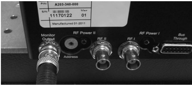
Figure 10: Electrical interface at the back of the SuperK SELECT
