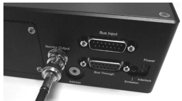
Figure 14: Power monitor electrical signal is available on the BNC connector
