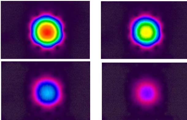
Figure 2: Near-field images of the fiber for optimum alignment (A) and gradually misaligned input beam (B-D). The output beam symmetry is maintained for all positions of the input beam and no higher order modes could be excited. The mode field diameter is  $32\ \mu\text{m}$ . The images are obtained on a CCD camera.
