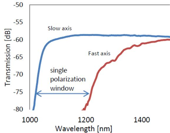
Figure 6: Transmission scan for the two polarization directions. The polarizing fiber structure yields a strong attenuation for the fast axis (y-polarization) for wavelengths  $<1200\text{nm}$ , while the slow axis (x-polarization) is well guided down to  $<1000\text{nm}$ .
