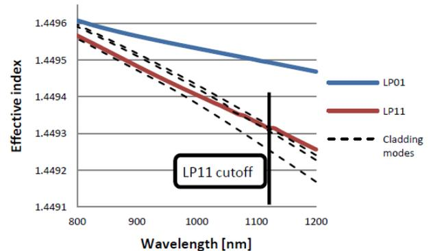
Figure 3: Simulated effective mode indices of the first 5 modes in a DC-200/40-PZ-Yb fiber. The  $LP_{11}$  mode exhibits a short-wavelength cutoff at  $\sim 1120\text{nm}$ , and the fiber is single mode for wavelengths below. The figure refers to the transverse (x-) polarized modes. The stress applying parts induce a strong birefringence, which lowers the effective indices of the corresponding y-polarized modes, which therefore are not guided in the wavelength range shown.
