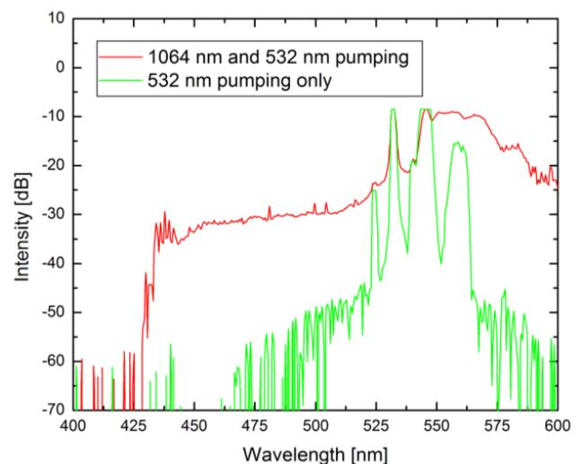
Figure 11: Generation of short wavelengths by dual pumping with 532 and 1064 nm in a NL-2.0-740 fiber.
