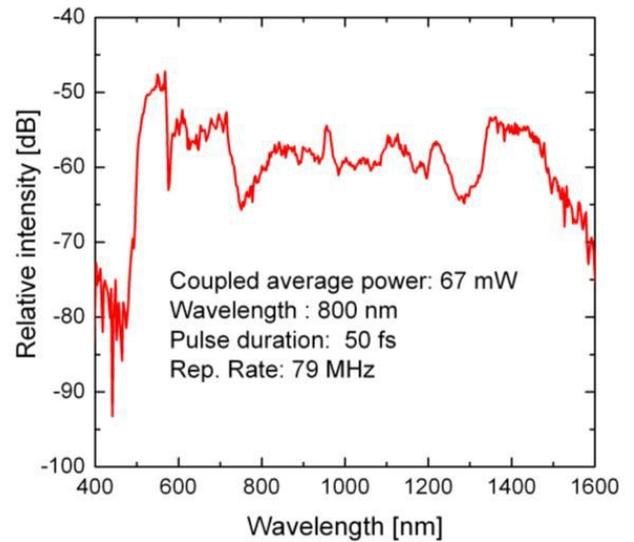
Figure 8: Octave-spanning supercontinuum generated in 1 m NL-PM-750 fiber.
