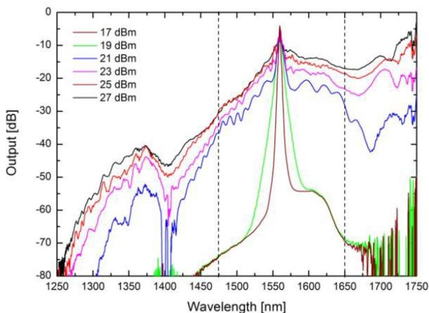
**Figure 12: Supercontinuum spectra from a NL-1550- POS-1 fiber pumped with a 2 ps 1555 nm source at six different pumping powers. The shown power levels are average coupled pumping power. Dashed lines indicate the two zero-dispersion wavelengths of the fiber.**
