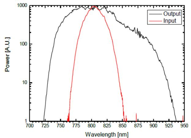
Figure 5: In- and output spectrum measured on 12.5 cm fiber pumped at 800 nm with 25 fs pulses (average power 53 mW and repetition rate 76 MHz). The fiber has normal dispersion and zero dispersion at 875 nm.
