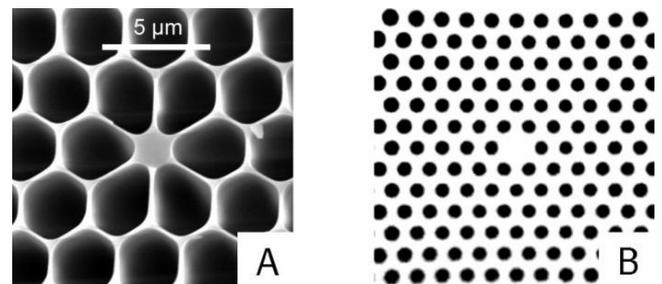
Figure 3 (A) SEM picture of a multimode fiber with zero dispersion at visible wavelengths. (B) Optical microscope picture of a single-mode fiber with zero dispersion at wavelengths around 800 nm. The relative hole-sizes are  $\sim 0.9$  and  $0.5$ , respectively. The pictures are shown on same scale.
