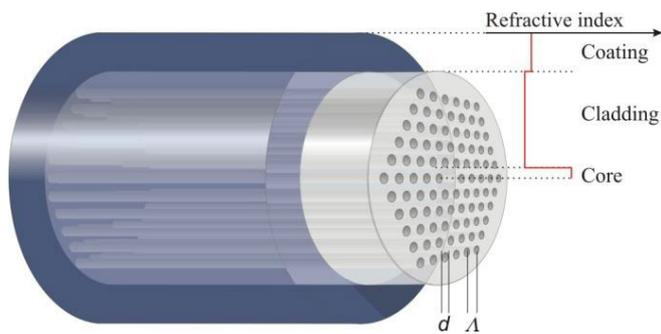
Figure 2: Schematic of the classical triangular cladding single-core photonic crystal fiber in which light is guided in a solid core embedded in a triangular lattice of air holes. The fiber structure is determined by the hole-size,  $d$ , and the hole-pitch,  $\Lambda$ . Like standard fibers, the PCF is coated with a high index polymer for protection and to strip off cladding-modes.
