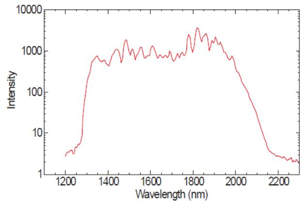
**Figure 13: 10m NL-1550-ZERO-1 pumped by an IMRA Femtolight B-60 (50mW, 1nJ, 110fs) at an average power of 22 mW. Measurements by Akira Shirakawa, Institute for Laser Science, University of Electro-Communications, Japan.**
