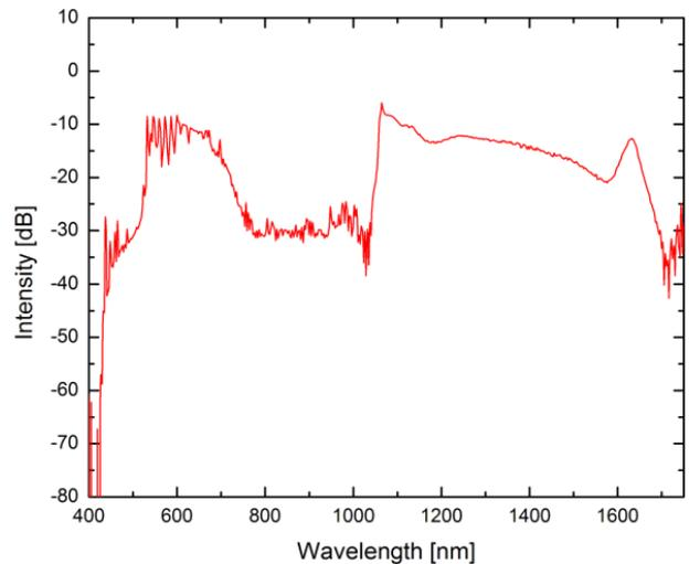
Figure 10: Supercontinuum generated in a nonlinear fiber with zero dispersion at 740 nm by simultaneous pumping with nanosecond pulses at 1064 and 532 nm. Measurements by Scott C. Buchter, Optical Fibre Group, Helsinki University of Technology [4].
