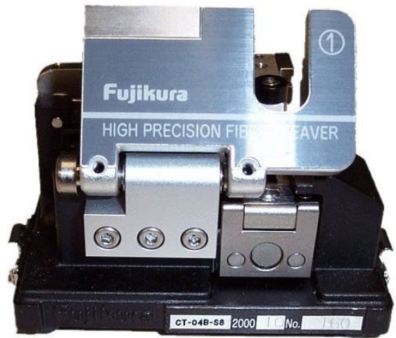
Figure 3: Fujikura CT-04 cleaver
