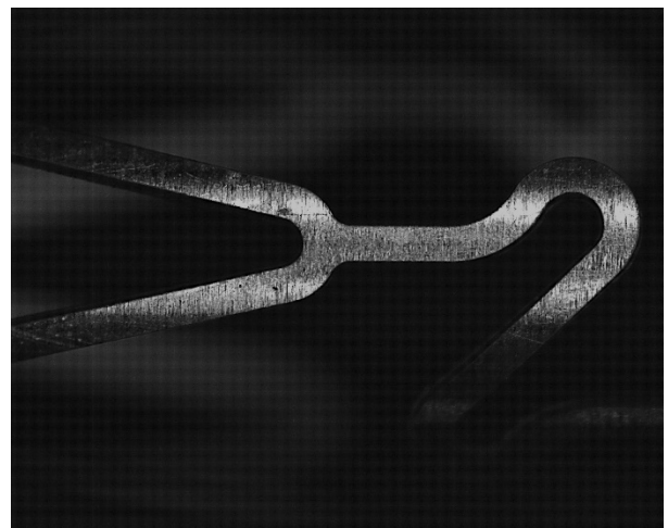
High quality stent machining of nitinol achieved using NKT Photonics' Origami XP laser.
